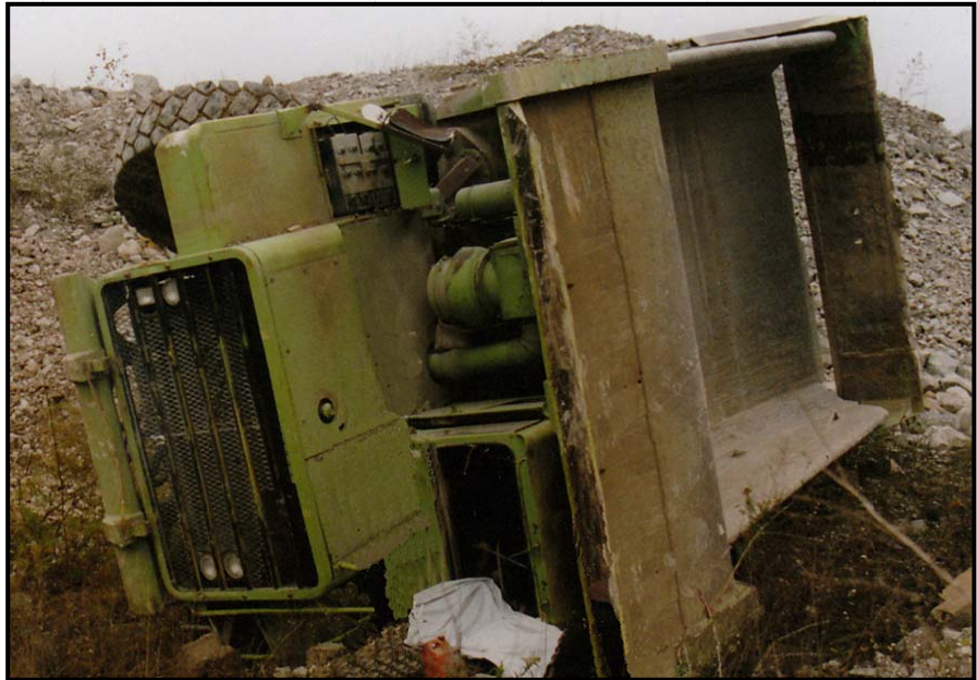
Photo 1 – Haul truck came to rest on its unbelted operator who was ejected or jumped.
