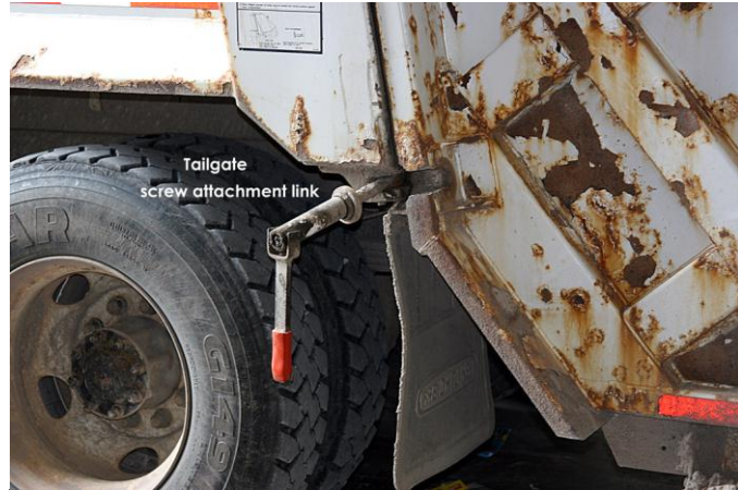
Exhibit 2: Attachment link that secures tailgate in closed position
