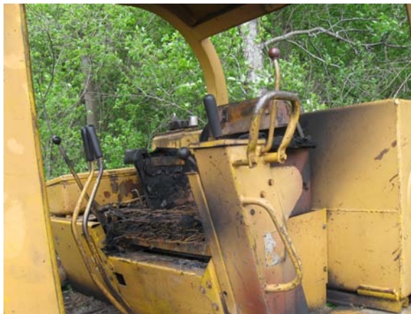
Exhibits 3A and B: Burned areas of the seat and battery compartment under the seat.
