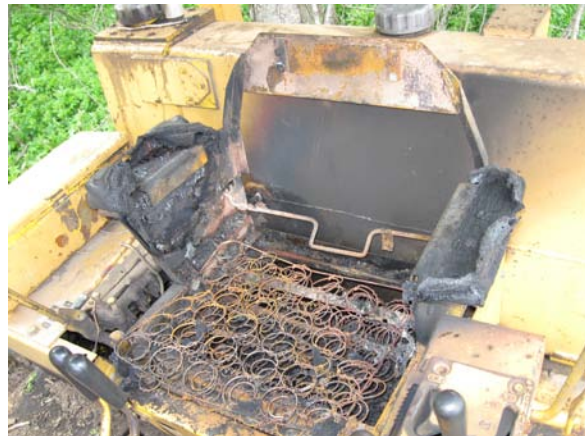
Exhibits 3A and B: Burned areas of the seat and battery compartment under the seat.
