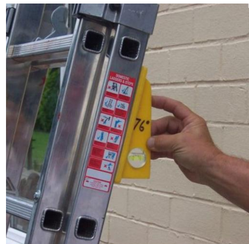
Exhibit 4. Proper height-to-base ratio and ladder angle to set up portable extension ladders
