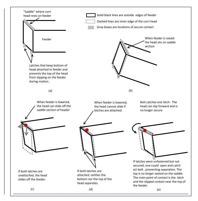
Post-Investigation: After the incident, the combine was taken to the dealer and a new locking mechanism (Centralized Header Latch Kit) was installed to replace the underside lever latches which had been the standard on these combines since the 1970's. The new mechanism has a
