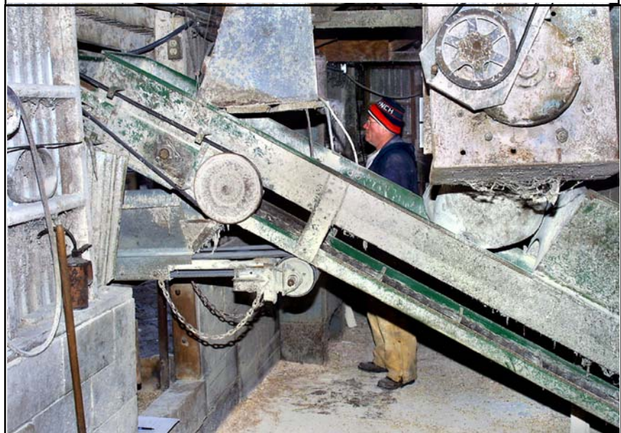
Photo 4 – View of conveyors from the doorway end of the shed, showing the farmer's normal work position, with the exposed ends of the horizontal conveyor at waist level.
