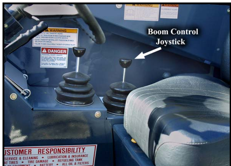
Photo 4 – View of cab area of a new identical forklift, showing position of the joystick which controls the boom.
