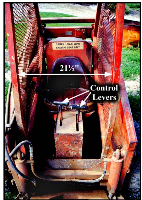
Photo 2 -- Front of skid loader showing narrow ROPS cage.
