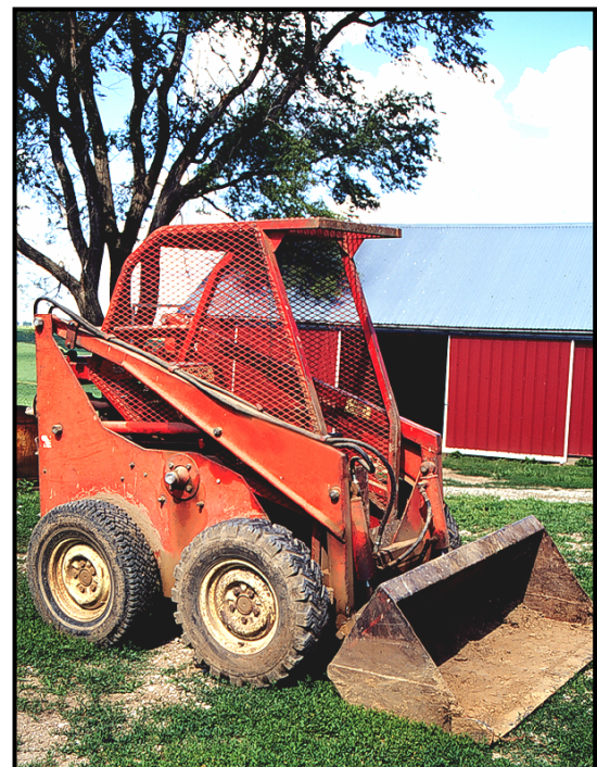
Photo 1 -- Old skid-steer loader with ROPS cage re-attached by new owner.
