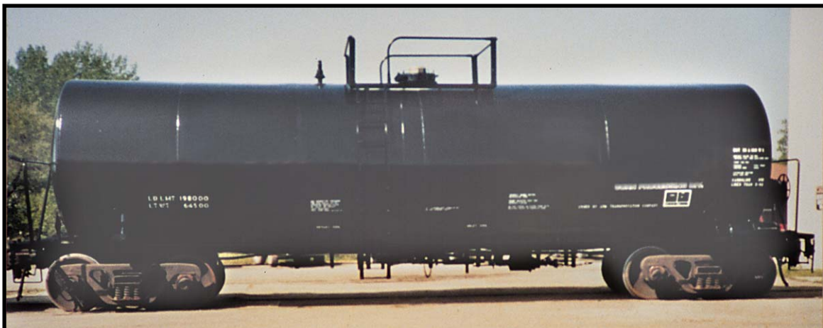
Photo 1 – Side view of similar rail tank car used to transport vegetable oil.
