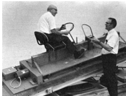
Dr. Berry (left) operates the IAM's "tilt table" that tested stability characteristics of small tractors and riding mowers; Dr. William McConnell (right) holds a steering tiller being tested by IAM researchers.
